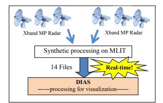
Fig. 3. Outline of acquisition XRAIN data processing on DIAS
