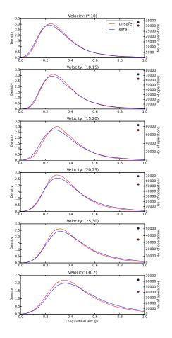
Figure 4. Density of longitudinal jerk during braking for various velocities
