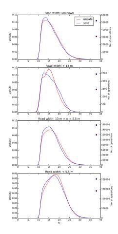
Figure 5. Density of yaw rate distribution during steering operation for various road widths
