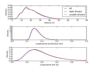
Figure 3. Distributions of braking operation variables
