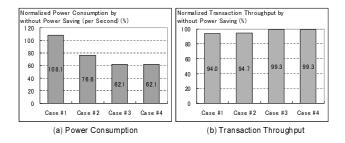
**Fig. 5.** Power consumption and transaction throughput under two disk drives for DBMS with the delayed write I/O method. The power consumption of disk drives is reduced by 37.9% with little transaction throughput degradation.
