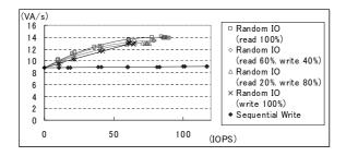
**Fig. 1.** Relationship between the disk drive power consumption and I/Os per second (IOPS). The power consumption of random I/O increases in accordance with an increase of IOPS. The power consumption of a sequential write is much less than that of random I/O.
