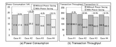
**Fig. 4.** Measured values of power consumption and transaction throughput (Two Disk Drives for DBMS). Proposed method reduces the disk drive power consumption by 23.1% with only 10% degradation of the transaction throughput.
