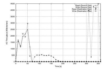
Figure 9. I/O Throughput (Runtime declustering from 1 to 8 disks)
