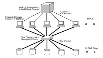
Figure 1. An overview of SAN-connected PC cluster pilot system
