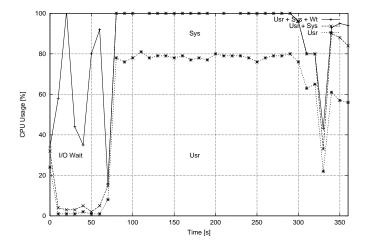
Figure 7. CPU usage (Runtime declustering from 1 to 8 disks)
