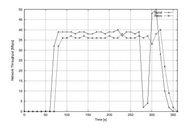
Figure 8. LAN Throughput (Runtime declustering from 1 to 8 disks)
