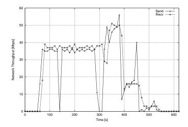
Figure 3. LAN Throughput (using 1 Disk)
