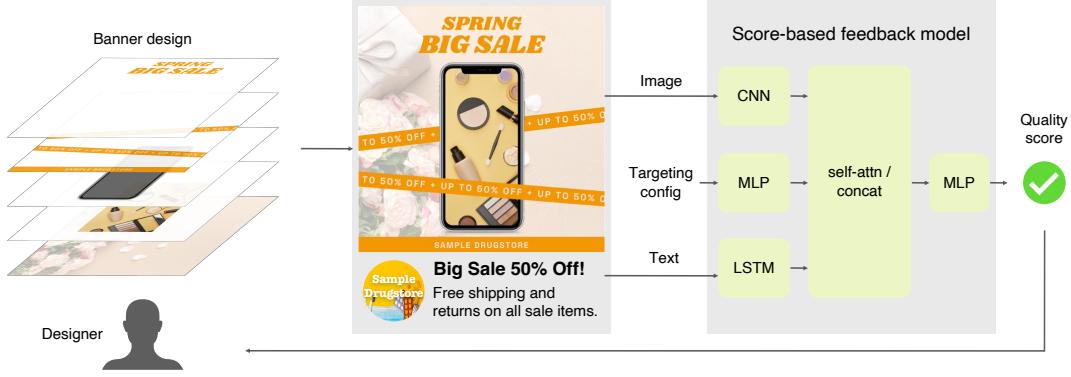
Figure 2: AI-assisted advertising creative workflow. The feedback model takes a banner image, associated text, and targeting configuration and predicts a quality score.
